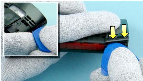
7) Release also the clips on the other side of the device.
