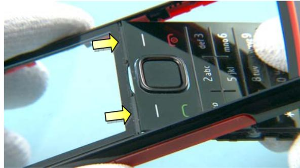
9) Make sure that the KEYPAD covers the bottom end of the A-COVER window shown by the arrows.
