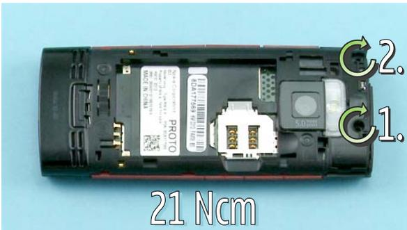
12) Tighten the two TORX + size 6 screws to the torque of 21 Ncm in the order shown.
