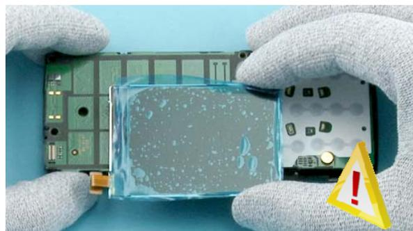
30) Remove the LCD DISPLAY carefully.
