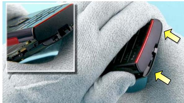
16) Open the remaining two clips on the bottom side of the phone.
