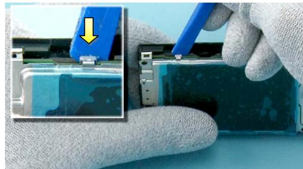
24) Release the second clip of the UI SHIELD with the SS-93.
