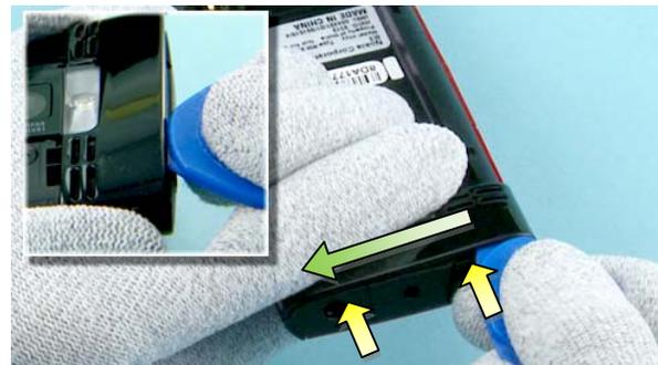
6) Release the two clips on the top side of the device by sliding the SRT-6 to the direction shown.
